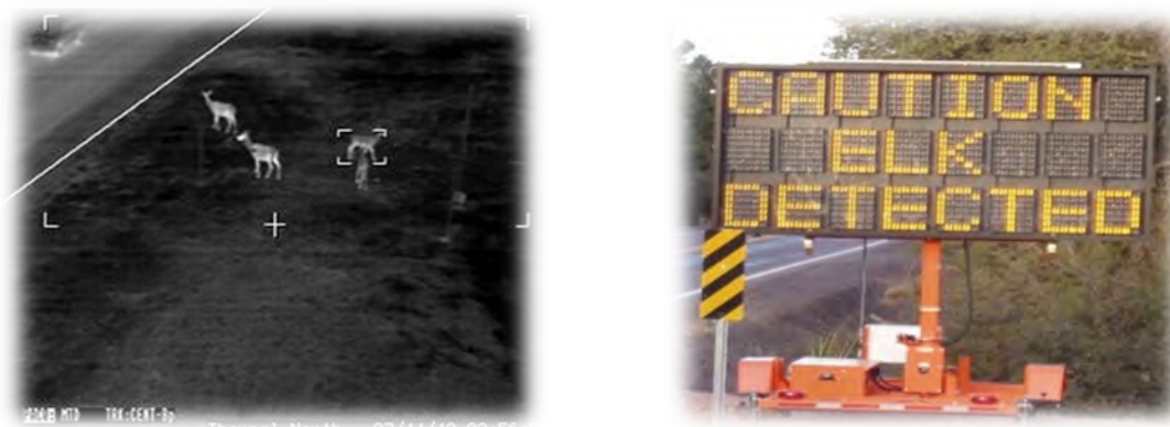
Figure 4-12. Example of thermal target acquisition software used to activate motorist alert signs (left) and sign activated when a
