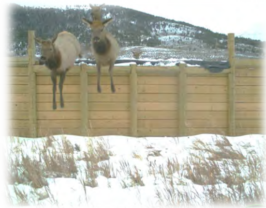
Figure 4-1. The monitoring for Colorado’s SR 9 had set performance measures. Cameras measured wildlife use of escape ramps. Photo Credit: Colorado DOT, Parks and Wildlife, and ECO-resolutions.
