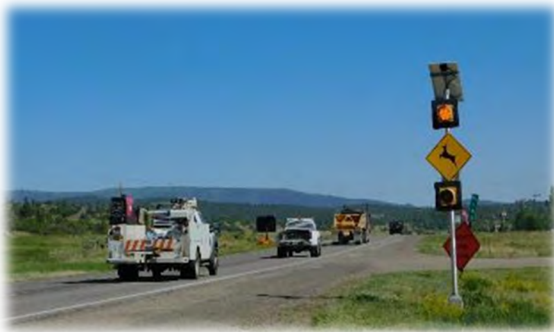
Figure D-50. Warning sign with flashing yellow lights in Chama, New Mexico. Photo Credit: P. Cramer.
